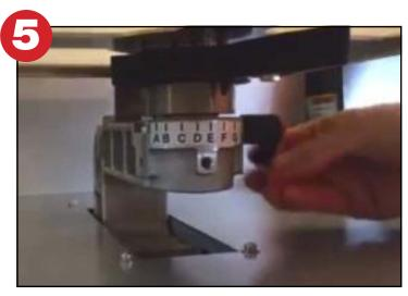
Step 5: Adjust the height of the platen to the desired position and tighten Locking Lever.
