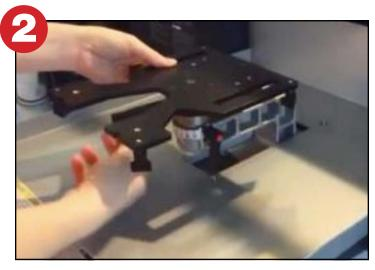
**Step 2:**Insert the T-Lock Base into the platen stem of the Brother DTG printer.
