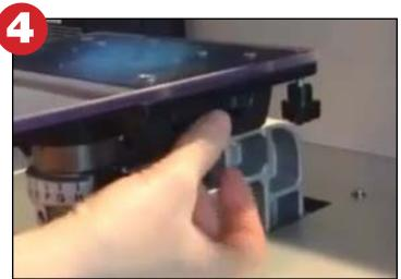
**Step 4:**Secure the Platen Insert by rotating the center piece in the T-Lock brackets.
