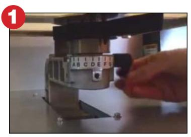
**Step 1:**Remove the Adult Platen by loosening the Locking Lever and lifting the platen straight up.
