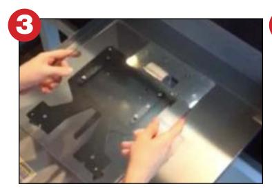
Install the T-Lock Oversized Insert so T-Lock brackets slide into the slots in T-Lock Base.
